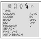
4 Press the V-/+ buttons to turn the SKIP function "ON".
